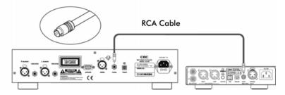
Connect to the COAXIAL terminal of any compatible digital audio device with a 75 Ohm COAXIAL (RCA) cable.
