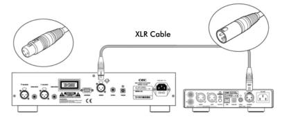
Connect to the AES/EBU terminal of any compatible digital audio device with a 110 Ohm XLR cable.
