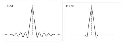
Needle Pulse response reproduced with Digital Filter set to FLAT and PULSE.
