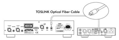
Connect to the TOSLINK terminal of any compatible digital audio device with an optical cable.
